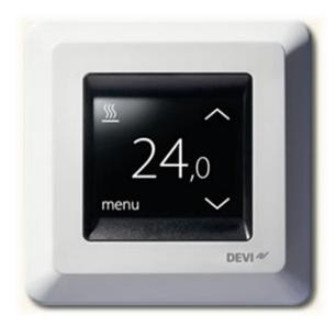
It is recommended that electric underfloor heating is controlled by a dual sensing room thermostat for each room or zone. The touch screen programmable room thermostat shown above that we offer can control electric underfloor heating in a room or zone up to a heat output of 3600 Watts. It has a floor sensor to limit the floor temperature and a built-in air sensor to control the room temperature. It is simple to use and can also be accessed remotely using a smart phone.
