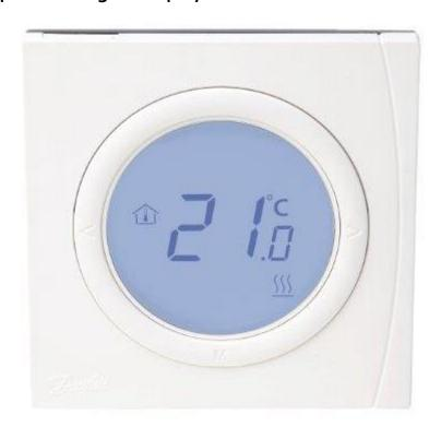
The WT-D is a 230V mains powered digital display room thermostat with large temperature display, back light and floor heating 'on' indicator as shown in the image above when the room thermostat is calling for heating to the room thermostat zone. This room thermostat can have an optional floor sensor connected to it to control the floor temperature. It requires an additional tamper proof night set-back sensor if a night set-back facility is required.
