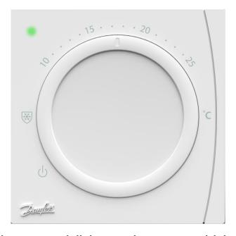
The WT-T is a 230V mains powered dial room thermostat with large temperature adjustment dial and indicator light as shown when the room thermostat is calling for heat. This room thermostat is a lower cost option to the digital display room thermostats. The WT-T room thermostat is air sensing only and cannot be connected to a floor sensor. It also requires an additional tamper proof night set-back sensor if a night set-back facility is required.
