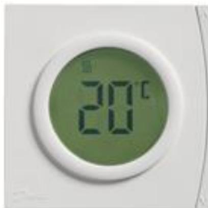
The RET2000B is a battery operated digital display room thermostat with a large temperature display, touch sensitive back lit display and heating 'on' indicator. It can be used as an optional room thermostat to be connected to the 24V SELV FH-WC wiring centre. It is air temperature sensing only and requires an additional tamper proof night set-back sensor if a night set-back facility is required.
